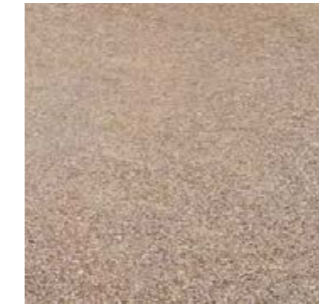
Spray tar and chip / Resin bound chippings Off-plot pedestrian and cycle path material, where high degree of flexibility is required.
