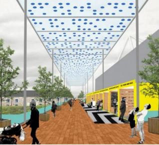
Elevated concourse canopy with pixelated solar collectors and cantilevered retail / maker / display booths to the eastern edge of the walkway.
