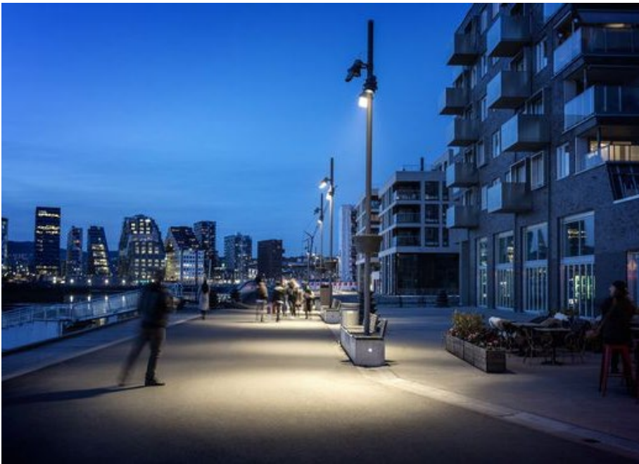
Bjørnvika, Oslo. Pole-mounted spotlights used to give direct illumination to key spaces around the dock edge, such as the Connaught Crossing.
